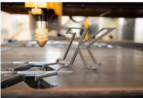
Picture: Optimal cutting results up to 60 mm with Kjellberg's new plasma power source K 200 (© Foto: Kjellberg Finsterwalde)
