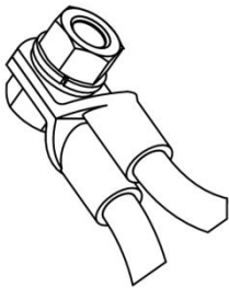
Fig. 19: If necessary, set the cable lugs of the cathode leads (connection 16) against each other.
