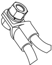
Fig. 19: If necessary, set the cable lugs of the cathode leads (connection 16) against each other.
