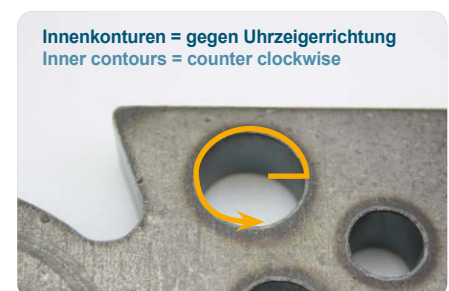
Schneidablauf Innenkonturen Cutting process for inner contours
